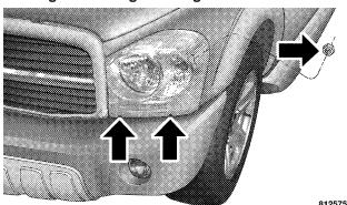
1. Remove the two bolts attaching the headlight to the inner fender panel.
